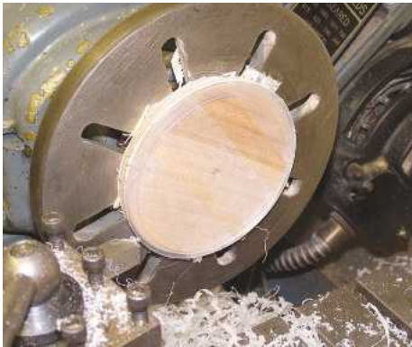
▲ Pic.22 Martin turned some thicker acrylic windows for the brass bezels...
